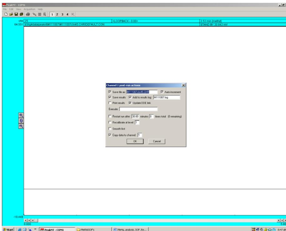
Modify both the “save file as” and “add results to log file” windows. In the “save file as” window adjust the folder and chromatogram names to represent present date and reset the CHR number to 00 (d:\hg6data1\peaknt\MMDDYY\MMDDYYCHRXX.CHR). The .log file also needs to be updated to represent the current date in the “save file as” window (MMDDYY.log).
